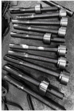
SLOTTED BOLT AND NUT FOR ADJUSTING MACHINES
